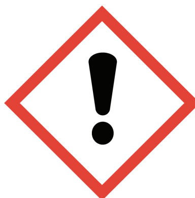
g – Irritant or harmful if swallowed, inhaled, upon skin contact or contact with the eye
